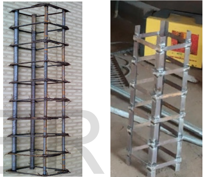
FIG 1 RCC COLUMN REBAR & PSC ARRANGMENTS
