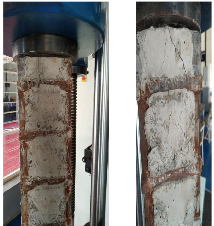
FIG 8 CRACKING OF SPECIMEN
